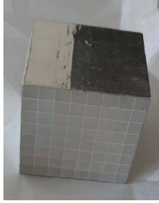
Figure 28. A 8 \times 8 matrix of LYSO/LSO crystals. To maximize light-gathering, the crystal matrix is coated with reflective foils.
