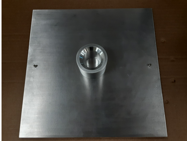
Figure 6: The jig used for aligning the inner conductor.
