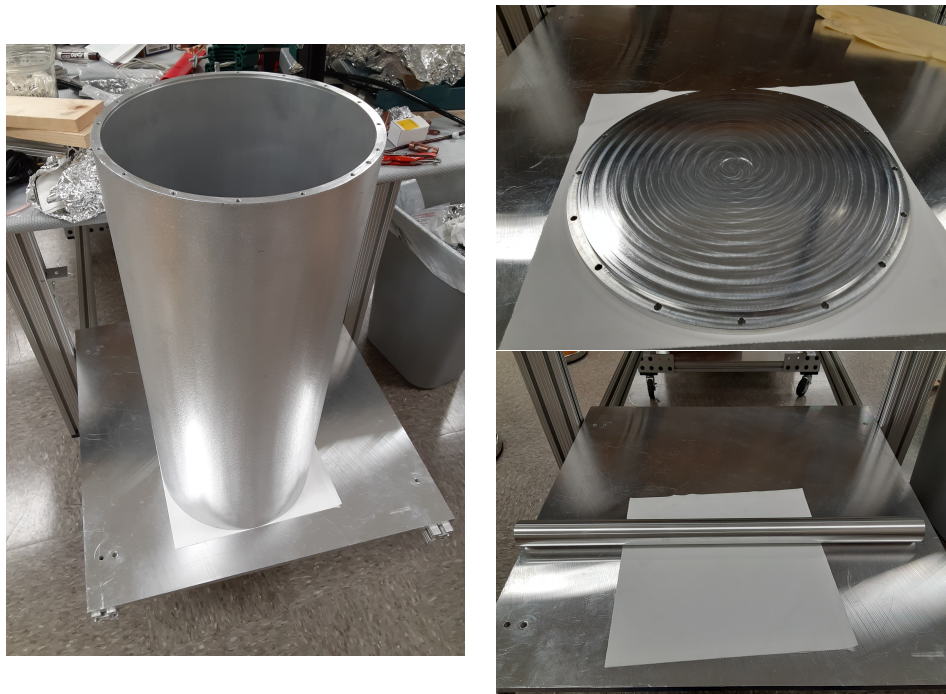
Figure 4: Aluminum outer conductor (left), bottom plate (right, top), and inner conductor (right, bottom) after machining.
