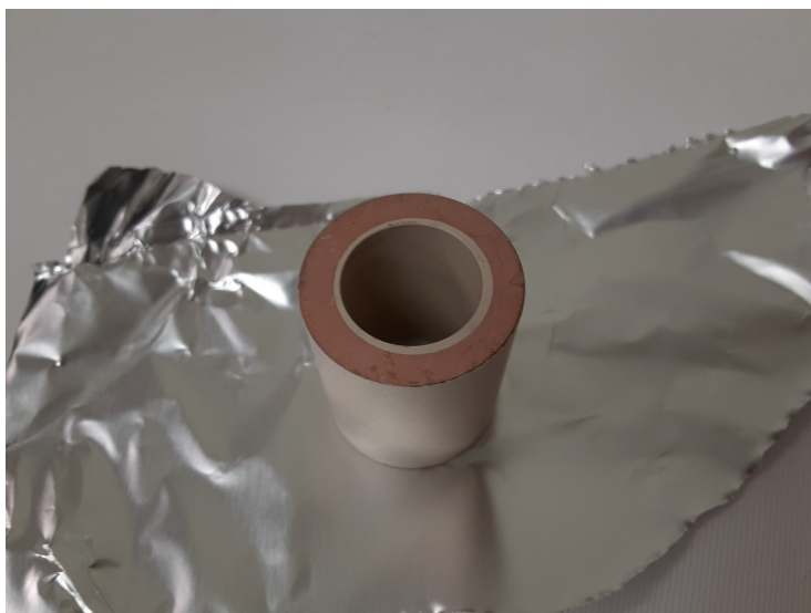
Figure 3: A ferroelectric tube after the ends were sputtered with copper.
