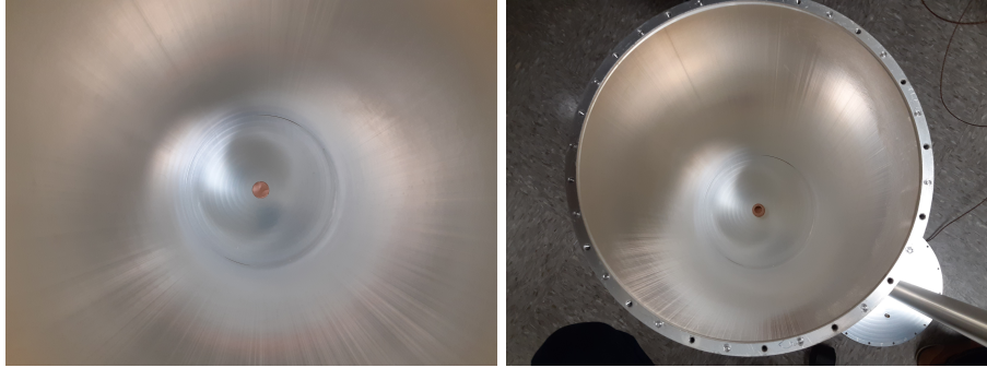
Figure 11: Photos of the copper foil disks placed in the bottom plate counterbore (left) and the ferroelectric tube placed on the foil (right).
