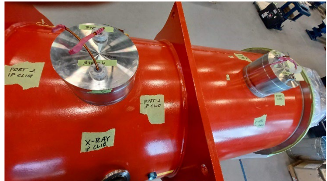
Fig. 18. CLIQ (left) and KMOD (right) warm head assemblies after being welded onto the vacuum vessel.
