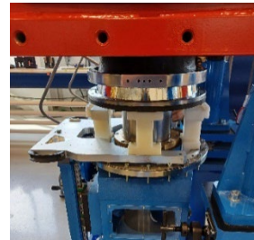
Fig. 12. Each alignment table includes provisions for lifting the support feet into the vacuum vessel.
