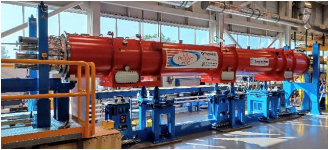
Fig. 14. The first HiLumi LHC Cryostat-Assembly after completion of assembly operations on the cryostat tooling.
