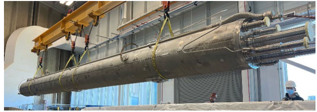
Fig. 5. The Cold Mass being transported to the cryostat tooling.
