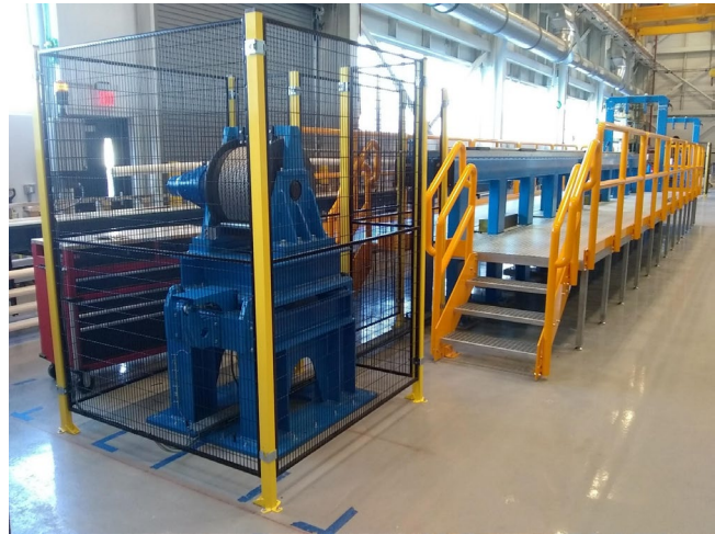
Fig. 1. The cryostat tooling, showing the decryostating winch, work platform, and assembly table.
