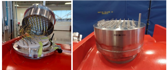
Fig. 17. Wiring of the IFS system, and after the IFS warm head assembly has been welded into place.
