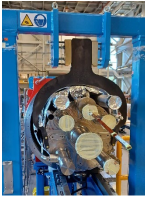
Fig. 3. Stabilizer installed on the end of the Cold Mass.
