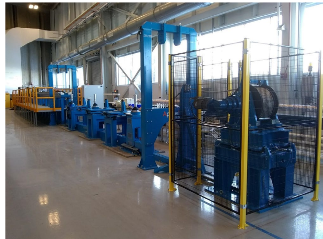
Fig. 2. The cryostat tooling, showing the cryostating winch, alignment tables, mechanical screw jacks, and stabilizer frames.
