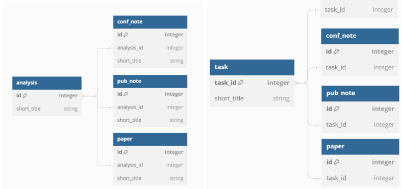
Figure 2. Model of denormalized schema Figure 3. Model of the refactored normalized schema
