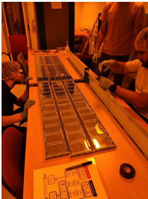
Figure 12: Assembly of supercells into PDS modules at CERN.
