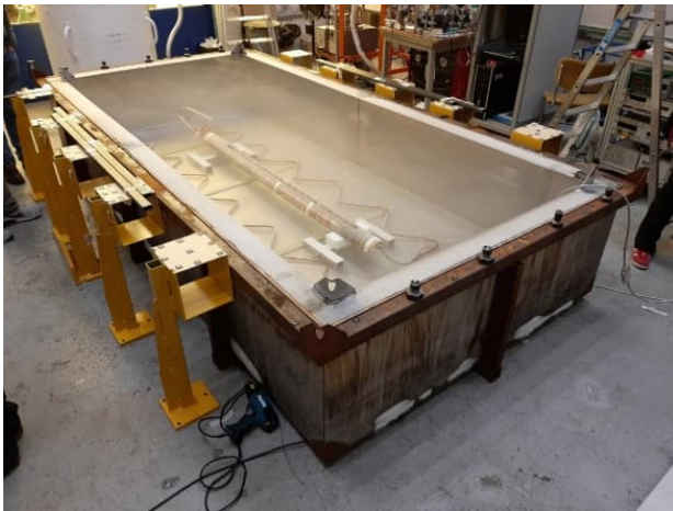
Figure 2: The setup for 11T short model coil cold test at CERN
