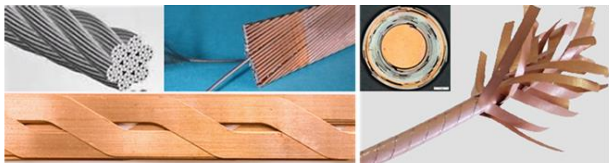
Figure 5.2. Rope (top left), Rutherford (top middle), Roebel (bottom left), and CORC ® (right) multistrand superconducting cables.
