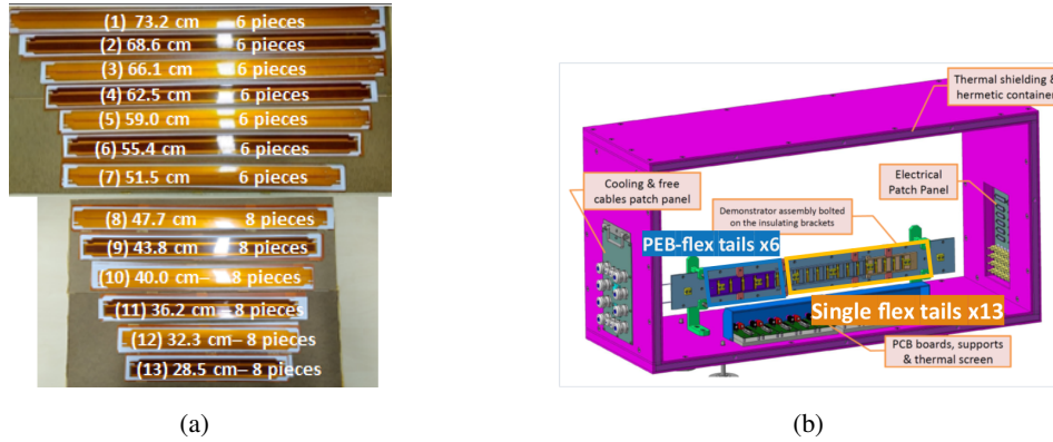
Figure 2. (a) 13 flex tail lengths of prototype A. (b) Sketch of the single readout-row demonstrator [2]. Copyright CERN for the benefit of the ATLAS Collaboration. CC-BY-4.0 license, re-used with permission [4].
