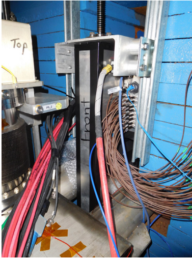
Figure 3. Photo of the RHICf detector, former LHCf Arm1, installed near the STAR interaction point. There is a structure allowing the detector to move vertically.
