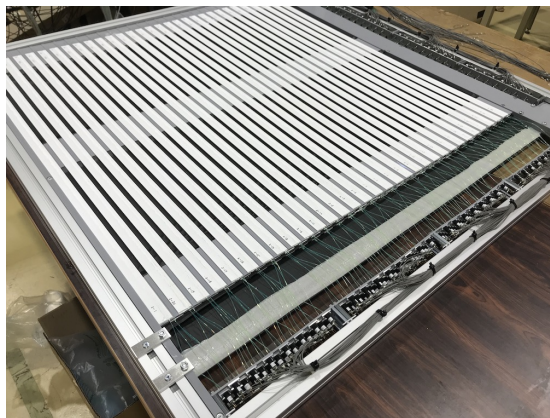
Figure 7: The scintillation tracker for the NINJA physics run. Scintillation light from each plastic scintillator bar is read out by the wavelength-shifting fibers and the MPPCs.
