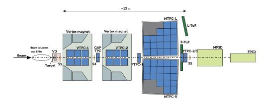
**Figure 2:** The contingency layout of the NA61/SHINE spectrometer with the idle MTPC sectors marked in grey.
