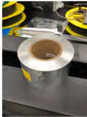
Figure 7 Heavy duty aluminium tape (0.25 mm thick), used to seal the flame shield
