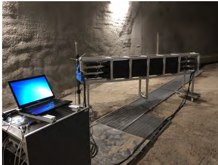
Figure 6: A photograph of the prototype MAPP-mQP detector and its readout system deployed in the UG1 gallery near to IP8
