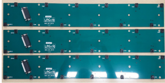
Figure 3. Set of 3 HVbus prototypes produced this year following the design from LPC Clermont Ferrand.
