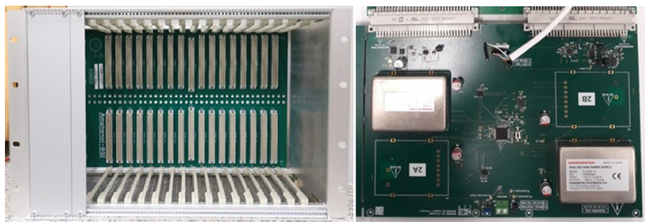
Figure 2. (left) Prototype of the crate for the boards. It has a midplane and the HVremote boards go in the back. (right) Prototype of HV supply board. It has two DC-DC Hamamatsu C12446-12 modules, each one able to supply 10 mA up to -1000 V.
