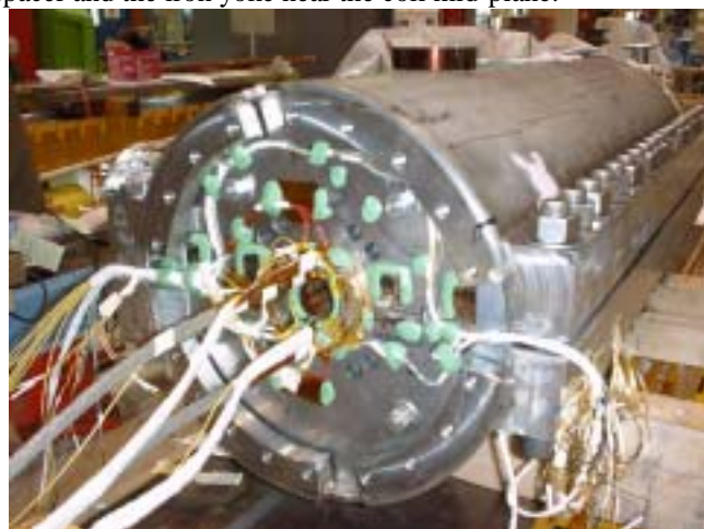
Fig.4. Dipole model HFDA05 (lead end, before installation of end plate and half-coil splicing).
