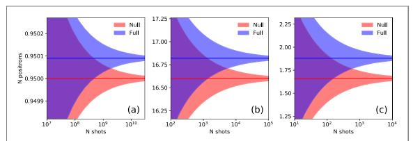
Figure 13. Mean number of positrons and  $2\sigma$  error against number of shots, for both full and null shots. (a) Predictions based on measurements made during the experiment. (b) Predictions based on optimum photon sources and the existing shielding configuration. (c) Predictions based on optimum photon sources, but with an extended setup that reduces the background noise by a factor of ten.
