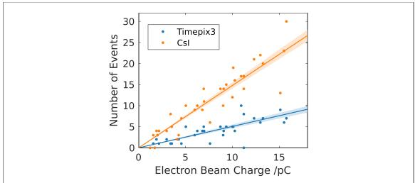
**Figure 11.** Variation of number of background events measured with electron beam charge on the Timepix3 and CsI detectors. Orange: CsI detector, Blue: Timepix3 detector. Shaded regions represent  $1\sigma$  confidence interval on the linear fit.
