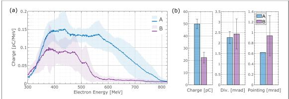
**Figure 3.** Properties of the electron beam used to generate the  $\gamma$ -ray photon source: (a) average electron spectra with standard deviation from mean (shaded). (b) Average electron beam properties with standard deviations (error bars). A (blue) and B (purple) represent the optimum beam performance and performance during commissioning, respectively.
