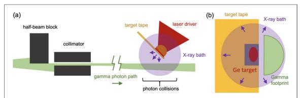
**Figure 2.** (a) Simplified view of the photon collision geometry. The tungsten half-beam block and collimator shape the  $\gamma$  beam to the desired profile before, much further downstream, colliding with the pre-expanded x-ray bath. (b) On-axis view of the overlap geometry. The x-ray bath radiates in all directions from the germanium target dot, providing a suitable particle-free collision volume for the D-shaped  $\gamma$  beam to pass through.
