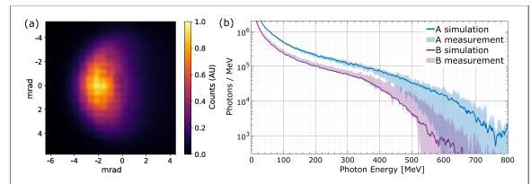
**Figure 4.** Properties of the  $\gamma$ -ray photon source: (a)  $\gamma$  beam profile example. The D-shaped footprint produced by the collimator and half-block shadows is clear. (b) Simulated  $\gamma$  spectra for both data sets (solid lines) and  $1\sigma$  interval of the first 10 spectra of the corresponding data sets measured with the  $\gamma$  spectrometer (shaded regions).
