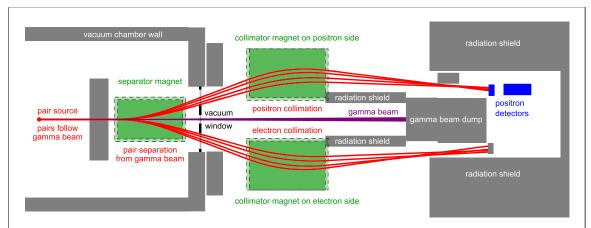
**Figure 6.** Overview of the AMS to transport generated pairs to the SPD. The combination of separator and collimator magnets was adapted for the energy range in this experiment by adjusting the length of the magnets and their separation. The electron and positron paths were adjusted to avoid the SPDs being directly exposed to radiation from noise sources inside the vacuum chamber (such as the electron source and convertor target).
