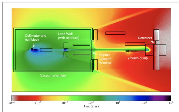
**Figure 10.** Combined photon and charged particle background noise flux throughout the setup. Simulated in Geant4. Lead walls shield the SPD location from direct sight lines to heavy noise sources such as the  $\gamma$  collimator and first lead wall aperture (labelled for clarity).
