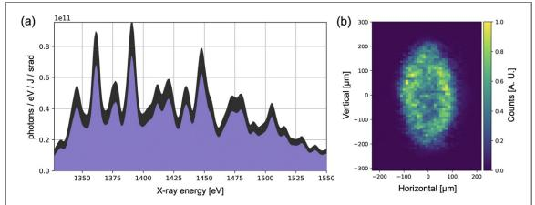
**Figure 5.** (a) Average x-ray spectra emitted by the germanium target. Measured using a thallium acid phthalate (TlAP) crystal spectrometer over 47 shots. The standard deviation is given by the black shaded area. (b) Example median-filtered x-ray pinhole camera image of the germanium target. The aspect ratio of the x-ray source closely resembles the f/2 focal spot.
