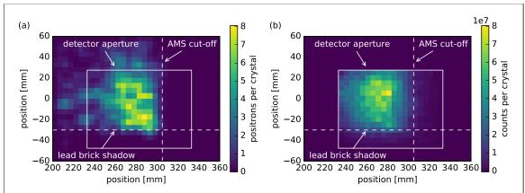
**Figure 8.** (a) The simulated positron hit map on the detector plane produced by the PTFE calibration target on a 9.2 pC<sub>r</sub> shot. (b) The measured detector response with the PTFE calibration target in the beam. The combined information from both images is used as a detector calibration.
