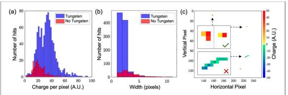
Figure 9. TimePix3 training data. Average charge per pixel (a) and cluster width (b) distributions for shots with and without an on-axis positron source (tungsten). The difference in the distributions with and without the positron source form the basis of a positron event specification. (c) Examples of the positron specification being implemented and rejecting non-conforming hits (highlighted with a negative colour value).
