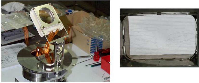
Figure 25: Pictures of a SEM grid assembly (left) and of damaged 50 µm tungsten wires (right)
