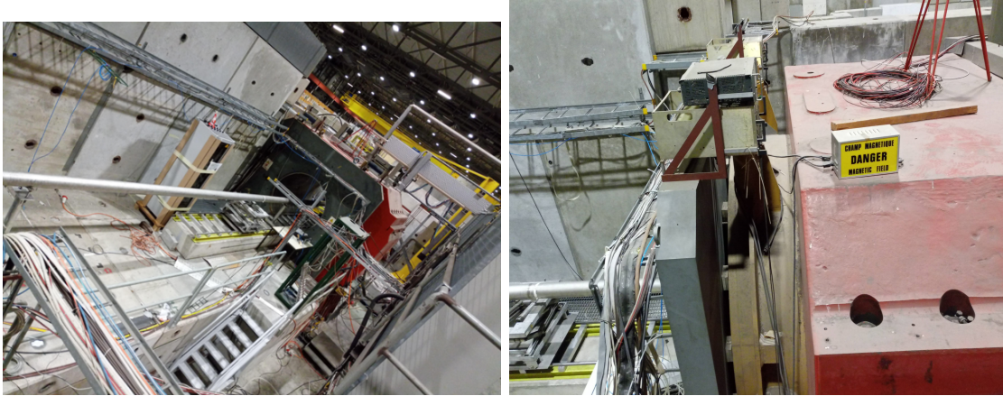
Figure 11: Left) View of the area around the MORPURGO magnet in the north area, as seen from the upstream side. The yoke of the magnet is in red. ATLAS rails are fixed on a support IPN (yellow) and on the magnet. Right) Zoom on the cables attached to the MORPURGO magnet.
