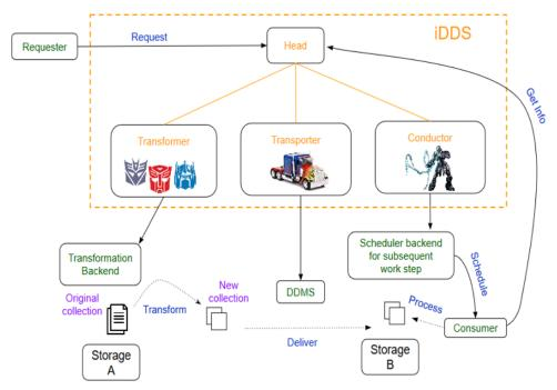
Fig. 2. A schematic view of the Intelligent Data Delivery Service.
