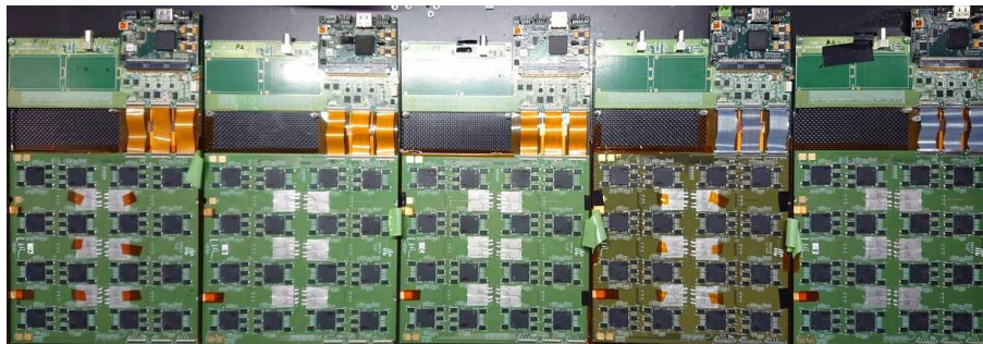
Figure 4: All slabs (FEV13) assembled in Kyushu University named from left as P1, P2, P3, K1 and K2
