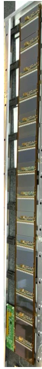
Figure 4: ITk barrel stave with 14 long strip modules. Each stave is 1.4 m long and 0.12 m wide.
