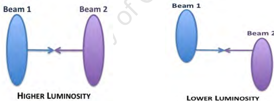
Figure 4.2: Schematic showing how luminosity can be adjusted by displacing the beam in the plane perpendicular to the beam axis.
