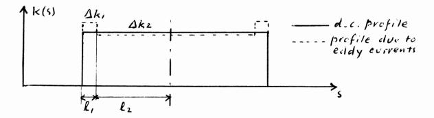
We call  $\triangle k_1$  and  $\triangle k_2$  the changes in focusing strength due to the eddy currents at the ends and inside. Due to the feedback from the reference quads we have
