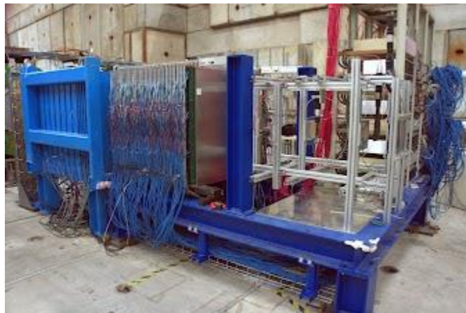
Figure 3. Photograph of the W-DHCAL (including main stack and TCMT) in the PS beam line, after cabling.
