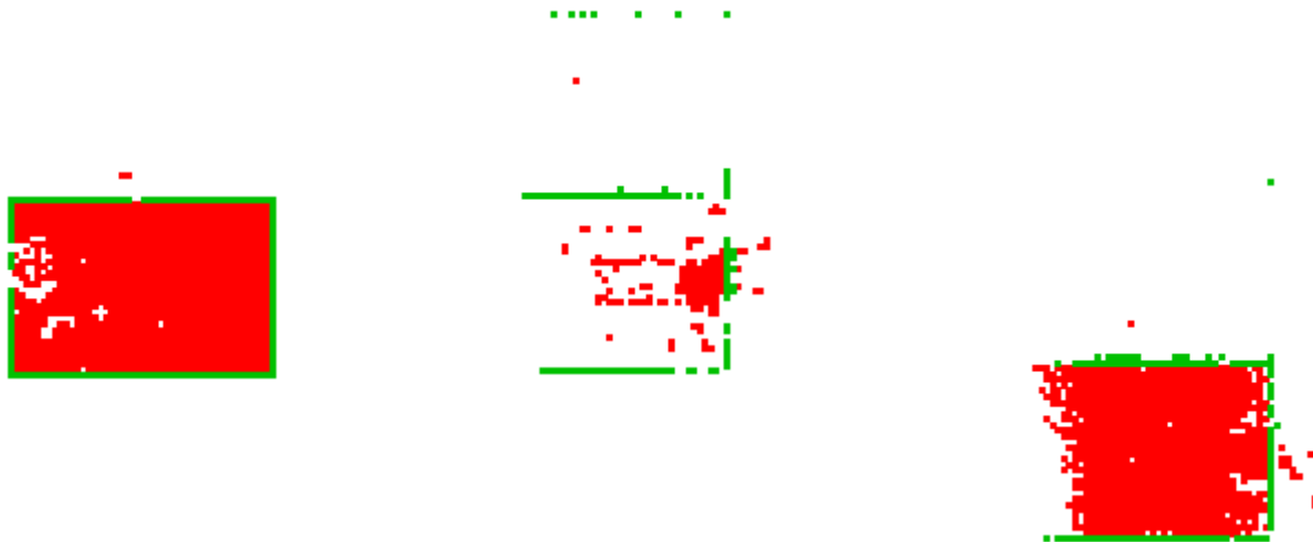
Figure 6. Hits in three different layers (from different events) showing un-physical hits related to the geometry of the front-end boards, so-called boxes. The hits on the inside (on the border) of the boards are shown in red (green).
