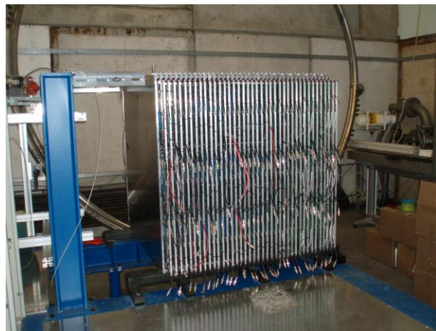
Figure 1. Photograph of the main W-DHCAL stack before cabling. The entire installation was placed on a platform, which facilitated the move from one test beam to the other.
