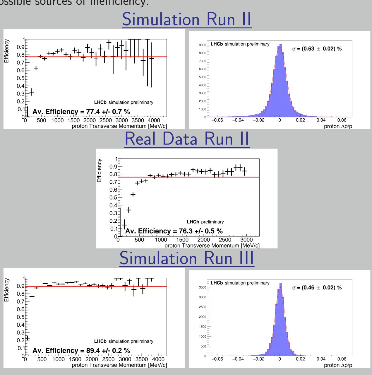
The new algorithms for the downstream tracking Run III has improve the efficiency and the momentum resolution [4]
