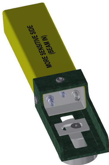
Figure 22: 3D drawing of the FIC BLM on its support, and the detector installed in the PSB.
