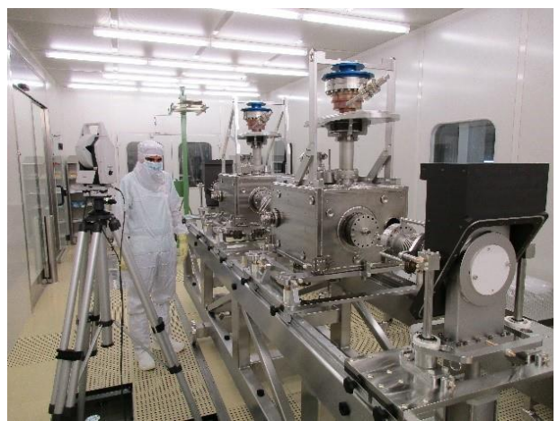
Figure 13: String assembly of the SPS-DQW dressed cavities in the SM18 facility.
