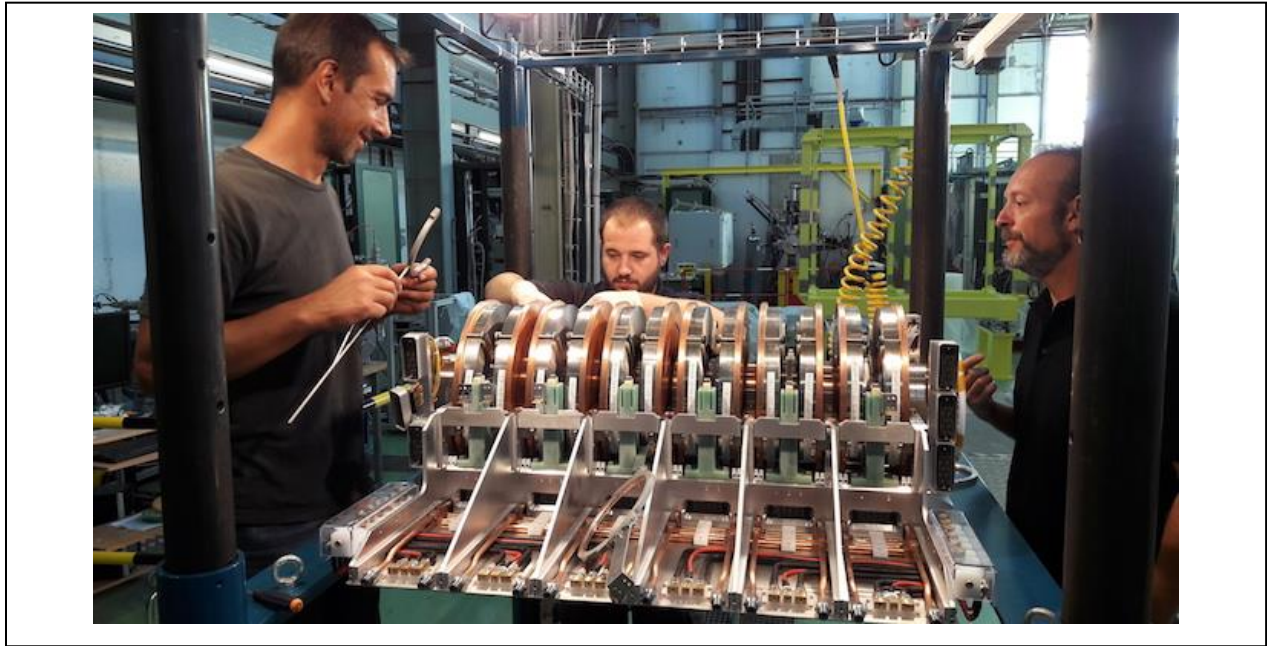
Figure 24: One of the new Finemet® based cavities of the PSB during its assembly at the RF workshop Meyrin
