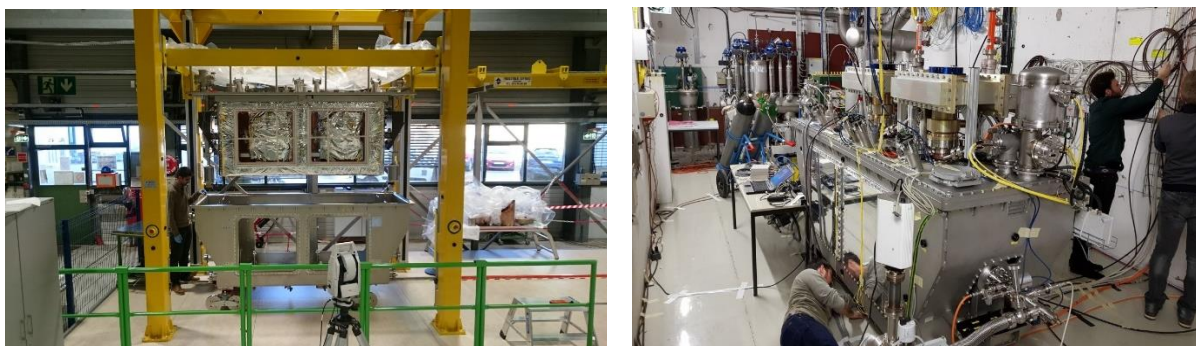
Figure 14: Cryostating of the 2-cavity string (left) and horizontal testing (right) in the SM18 facility
