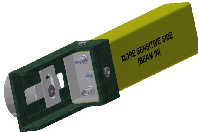
Figure 21: 3D drawing of the assembled support together with the FIC BLM detector.
