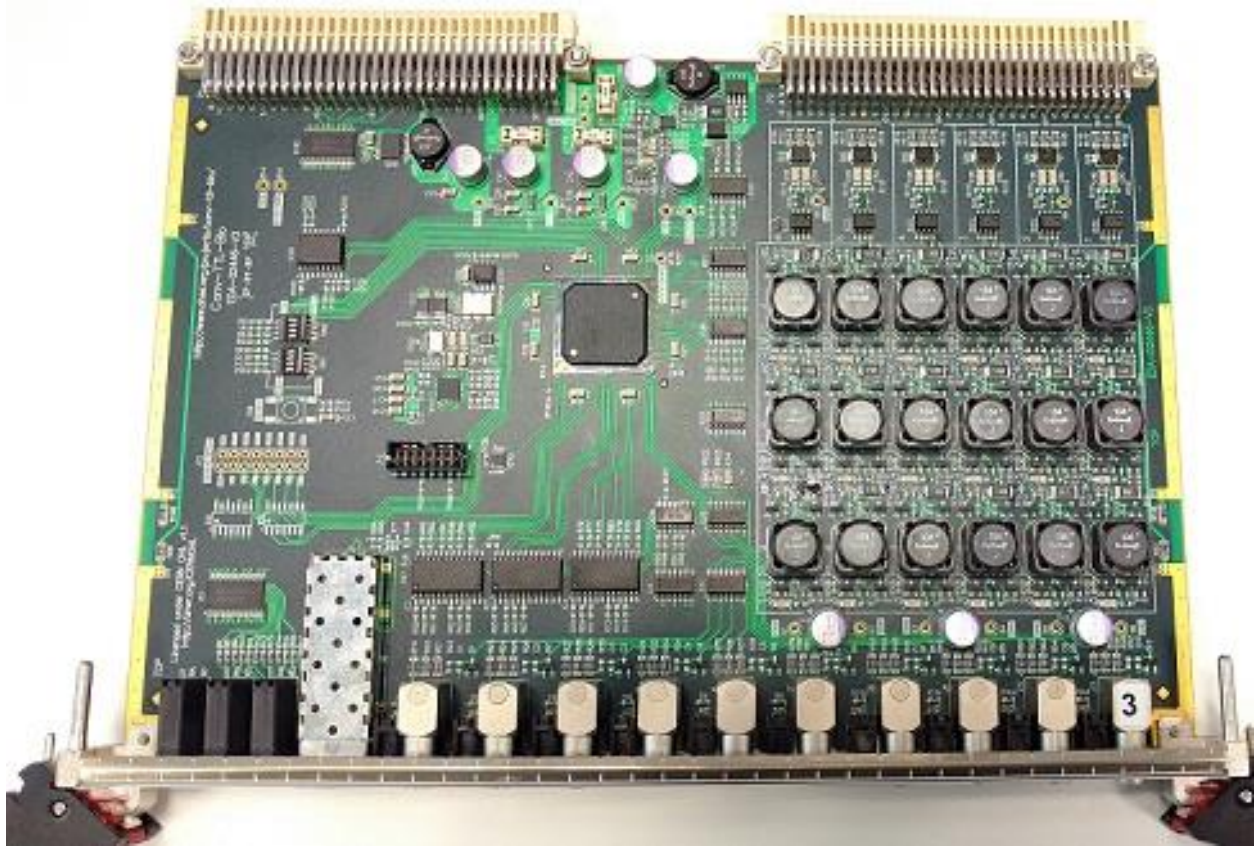
Figure 52: The new TTL-blocking converter module.
