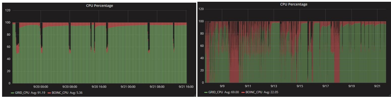
Fig. 1 CPU utilization on one node over one day (left) and two weeks (right). Green: grid jobs, red: BOINC jobs
