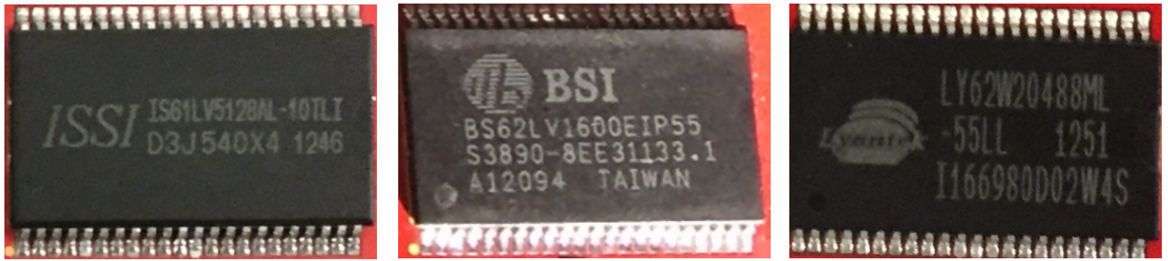
Figure 25: SEL-tested memories: ISSI 1246 (Left), Brilliance 12094 (centre), Lyontek 1251 (Right)
