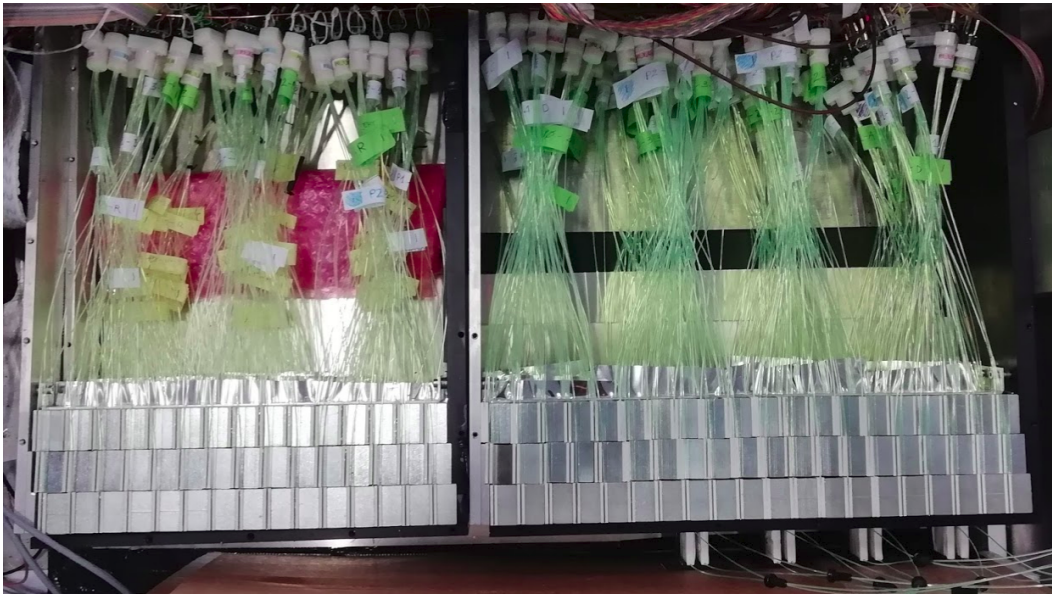
Figure 6: (Top Left): The prototype exposed at the CERN-PS T9 particle beams. The calorimeter is composed of an inner part (bottom part of the picture) made of seven calorimetric blocks and a 60 cm long “hadronic” block in the outer part (upper part of the picture). The system was mounted on a tunable mechanical cradle to record particles impinging at different angles. (Top Right): distribution of the tracks’ impact parameters on the front side of the calorimeter as predicted from Silicon tracking chambers using the 5 GeV beam. The layout of the calorimeter is superimposed: each square represents a 3 \times 3 \text{ cm}^2 UCM. (Bottom): The lateral readout prototype tested at the PS-T9 area in September 2018. The t_0 -layers are also visible in the bottom right part of the picture.
