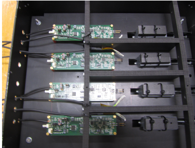
Figure 2: Setup of the gain stabilization measurements inside the black box. The green circuit boards host the preamplifiers and signal readout. The black cable attached is the signal cable. Each SiPM is inserted into a connector on the left-hand side. The Pt1000 sensors positioned near the SiPM are clearly visible. The clear fibers transporting the blue LED light run inside the black distance-adjustable foam boxes on the right, which were mounted precisely to illuminate the SiPM uniformly.
