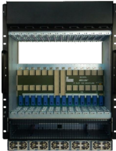
Figure 1: A 14 slot ATCA shelf with integrated redundant AC-DC power supplies.
