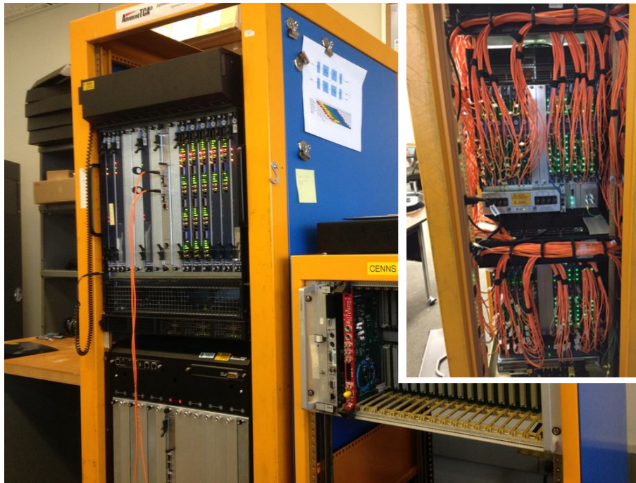
Figure 13: The Pulsar2 test stand at Fermilab. The upper ATCA shelf (COMTEL) is for Pattern Recognition Boards (PRBs) and the lower shelf (Schroff) is for Data Source Boards (DSBs). The short rack contains a VME crate and TTCcx board. Inset: the rear of the rack showing 100 QSFPP+ cables connecting the two ATCA shelves.
