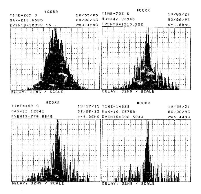
Fig. 5. The dependance of the number of photocount pairs from time interval between photocounts for the short electron bunch (150 ps).
