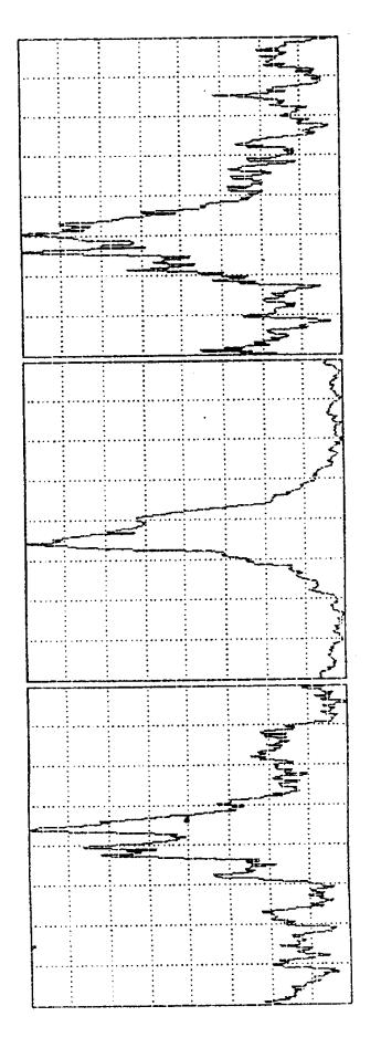
central line and sidebands is 1 kHz. Horizontal scale is 6.25 Hz/div. Amplitude of the central line corresponds central line, right - upper sideband. Distance between caused by near the 17th harmonic of synchrotron oscillations. Left - lower sideband, center one electron approximately as 5:1 to the sidebands amplitude. therevolution frequency for Fig. 6. The sidebands
