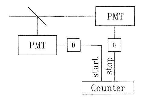
Fig. 2. Layout of the time interval measurements.
