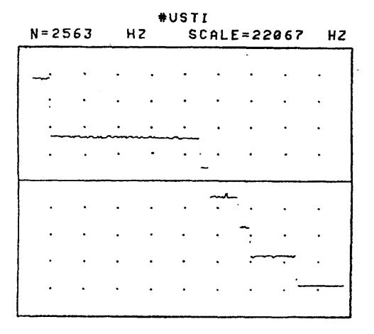
Fig. 3. The dependence of the counts rate from time. One step corresponds to the blow out of one electron. (Vertical scale is 22 kHz, horisontal scale is 2560 seconds).
