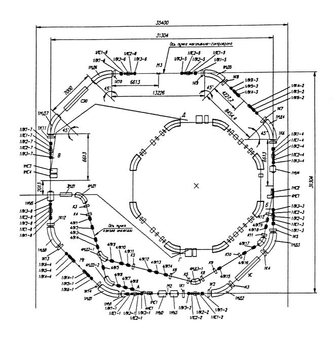
Fig. 1. The INR (Kiev) Storage-Accelerating Complex
