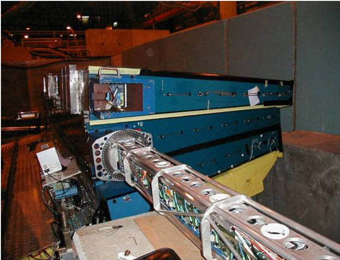
Figure 1.13 A super drawer being installed inside the module's girder.
