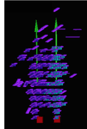
Fig. 2. One example of the correct reconstruction of two overlapping electromagnetic showers initiated by 4 GeV positrons separated by 2 cm using Garlic program.
