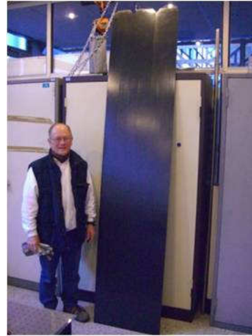
Figure 4: One layer molded (3 alveoli, L = 2.490 m, wall thickness 0.5 mm).
