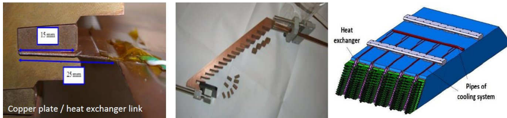
Figure 9: Left: Design of connection of heat exchangers with one copper drain extremity. Middle: heat exchanger for 15 \times 2 connections. Right: location of cooling system on one Si/W ECal barrel module.
