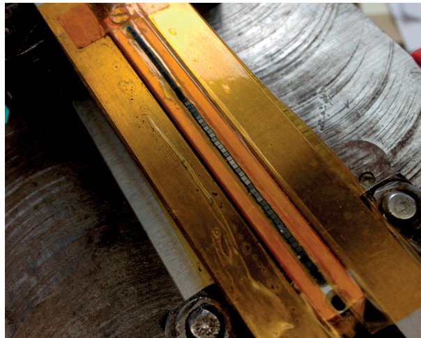
Figure 5.7 – Fibres on the mirror holder during polishing with sandpaper. Note: there are metallic accessories on the sides of the holder in order to guarantee mechanical stability during the polishing. The orange tape helps avoiding the creation of metallic dust that could harm the fibres.
