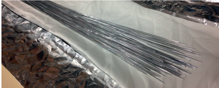
Figure 3.5 – Plastic scintillating fibres coated with a 100 nm aluminium layer. Note: it can be appreciated how the coated fibres do not scintillate in the presence of ambient UV light, in contrast with the uncoated fibres of fig. 3.1.
