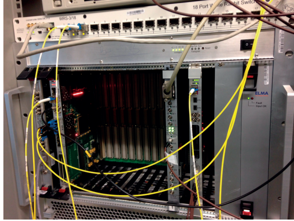
Figure 7.16 – VME crate in the control room hosting the VFC board for the XBPF event acquisition (second module from the left) and the TDC for the Time-of-Flight measurements (fourth module from the left). The White Rabbit switch that provides a common reference clock is standing on top of the crate.
