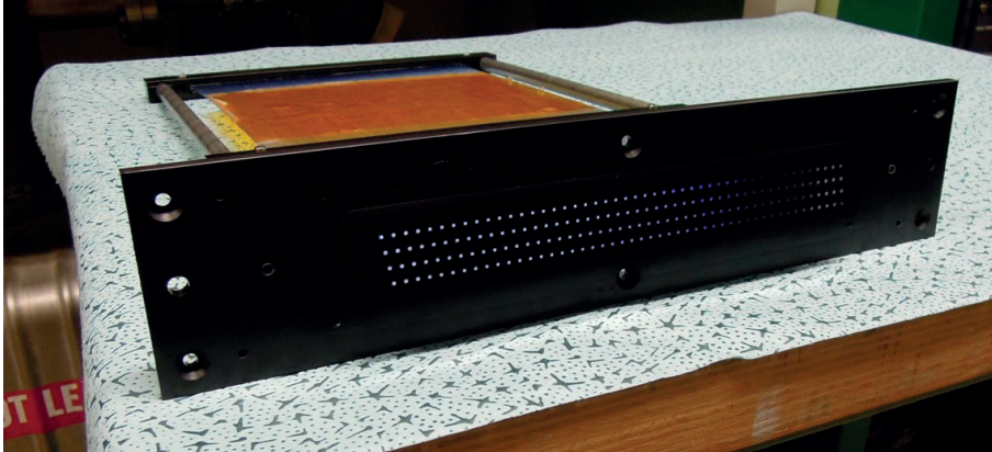
Figure 7.5 – Fibre connector where the scintillating fibres are coupled to the SiPM.
