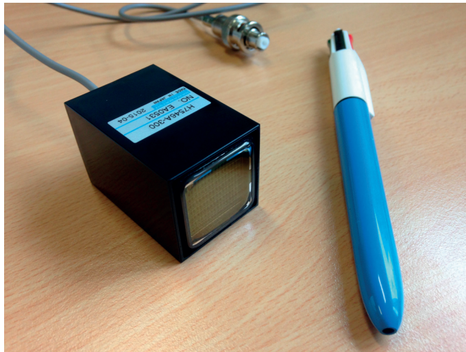
Figure 4.2 – Multi-Anode Photomultiplier H7546 from Hamamatsu.
