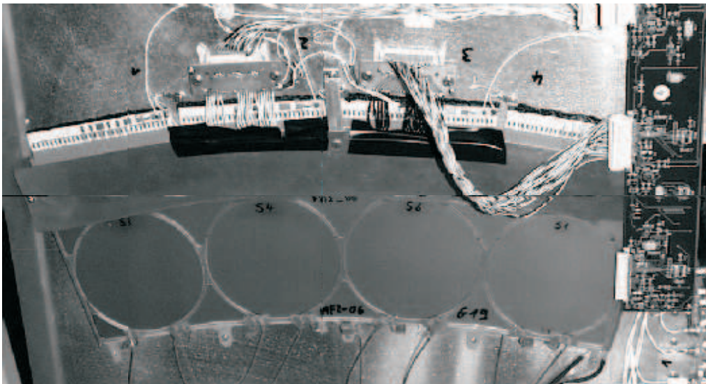
Figure 5.3: Multi substrate MSGC+GEM detector module mounted on a support plate with electronic readout and power supply boards.
