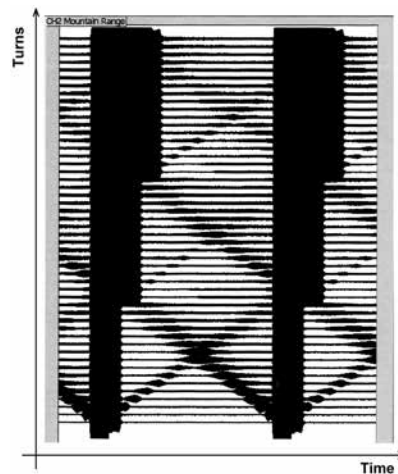
Figure 11.23: COLDEX MD2: 1% of the beam is uncaptured at the first batch injection and leads/lags in the longitudinal phase space, as measured by the SPS Mountain Range 200 MHz RF pick-up.
