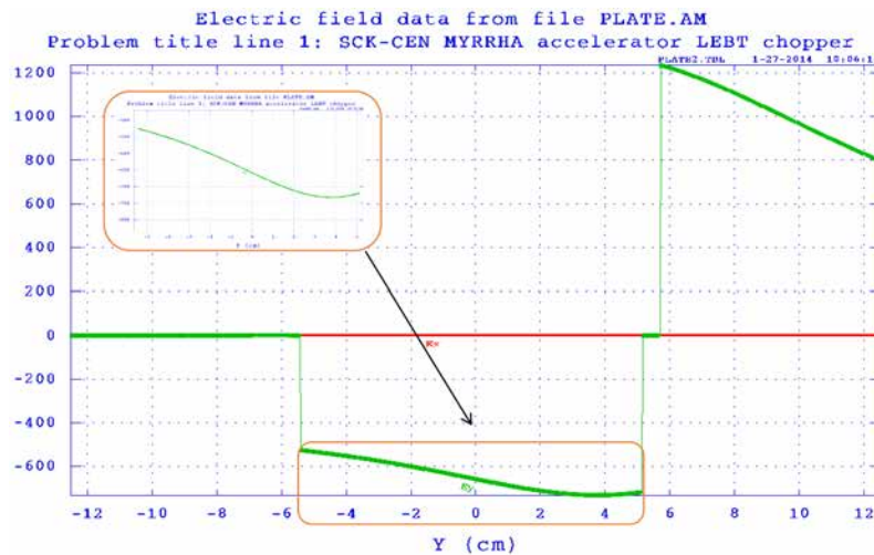
Figure 6.22: Horizontal E_x and vertical E_y electric field components, along the y axis in the transverse xy plane, of MYRRHA LEBT chopper, nominal position.
