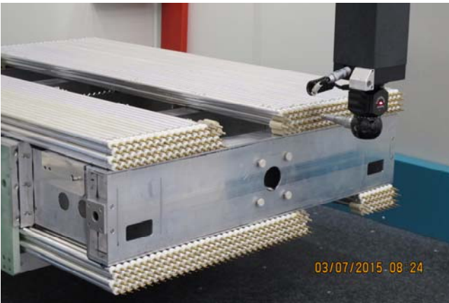
Fig. 4: The external reference surfaces of the endplugs allow for measurement of the relative wire positions of all drift tubes in an assembled chamber using a commercial coordinate measuring machine.
