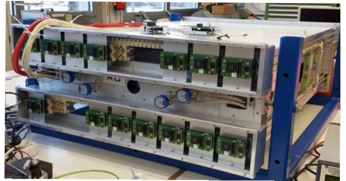
Fig. 6: A completed sMDT chamber for installation in the feet regions of the ATLAS barrel muon spectrometer in the LHC winter shutdown 2016/17 with mounted readout electronics boards ready for cosmic ray test.
