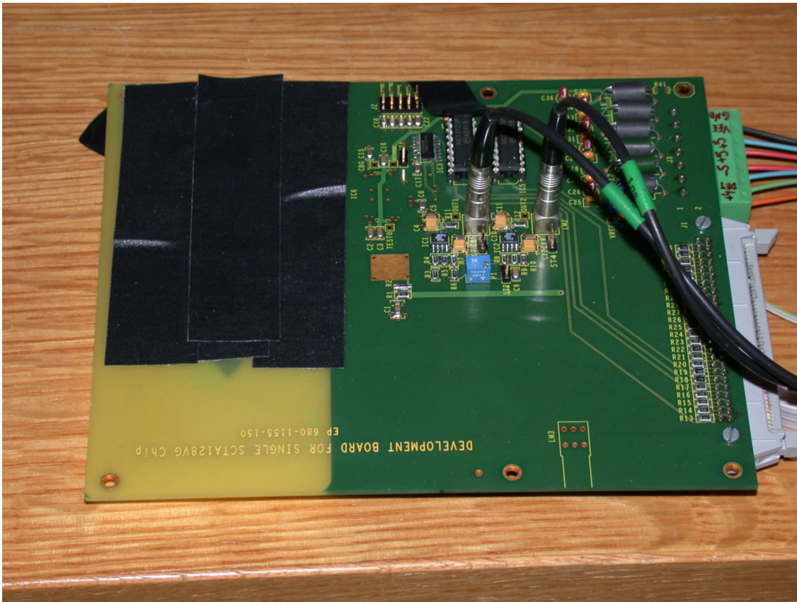
Figure 6.8: Single chip tests (the chip is in a protected space underneath the PCB).
