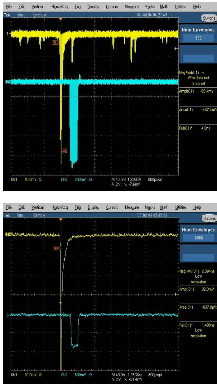
Figure 2.9: Signals obtained during a test beam at CERN. The top (bottom) figure shows the signal obtained from the plate with Y-Shape (HE and O Shape) fibers.
