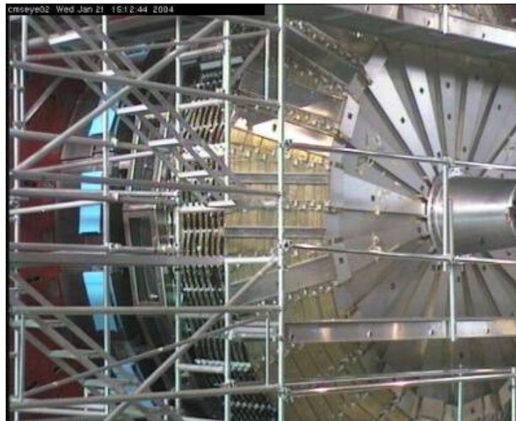
Figure 2.1: Mounting of the HCAL endcap (HE) on the disk of the endcap yoke.
