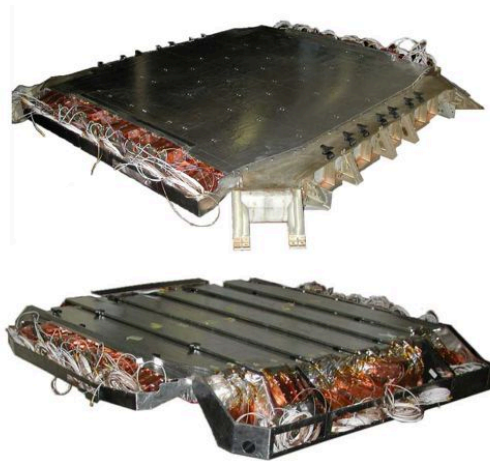
FIGURE 2.7: The upper and lower ToF assembled before the final shielding. The scintillator paddles, the bent light guides and the PMT are exposed.
