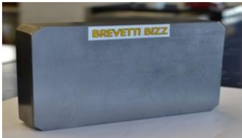
Figure 1.7 MoGR sintered plate.
