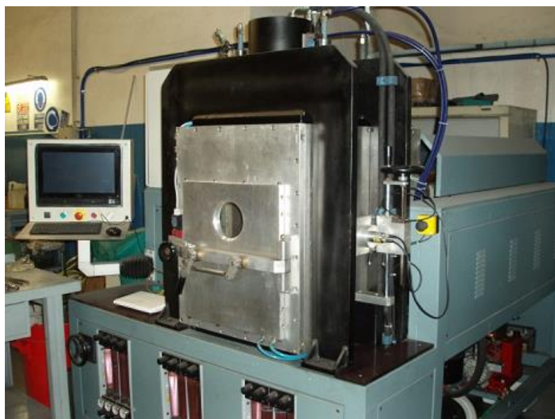
Figure 1.5 Hot-pressing machine at BrevettiBizz.
