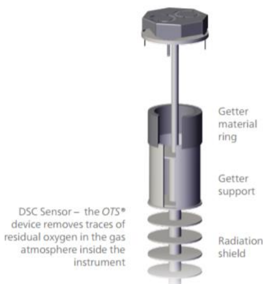
Figure 3.8 Sample holder and OTS system.
