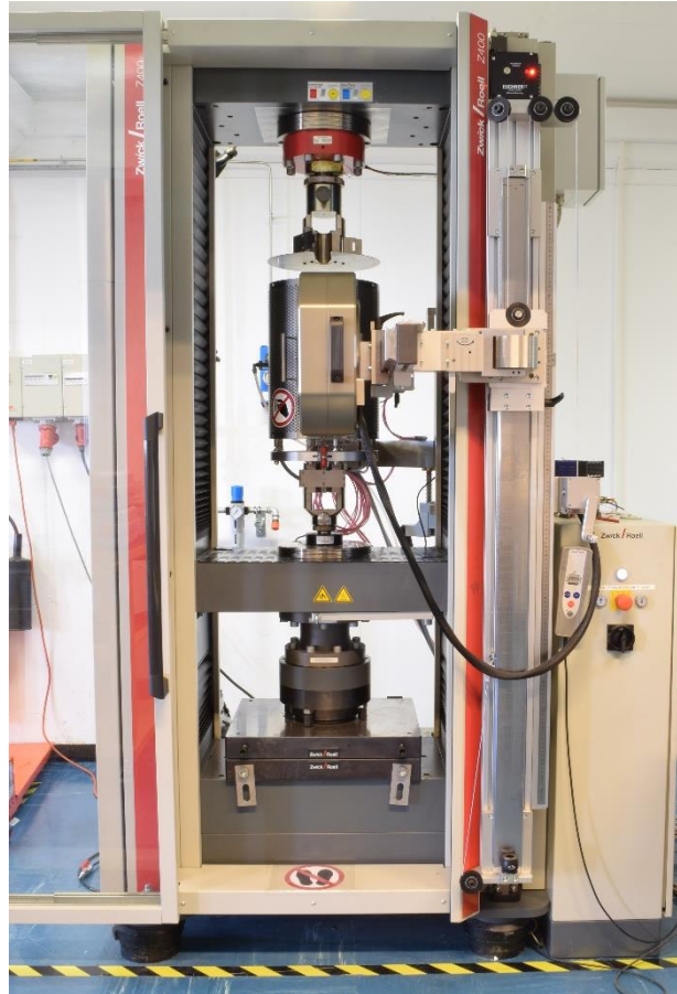
Figure 3.9 Universal testing machine Zwick Z400.
