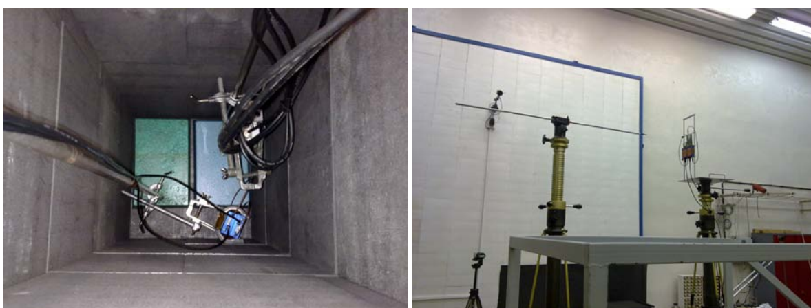
Figure 59: Calibration set-ups in CMI: A graphite prism with thermal neutron field (left) and a rod with a fast neutron source tip (right).
