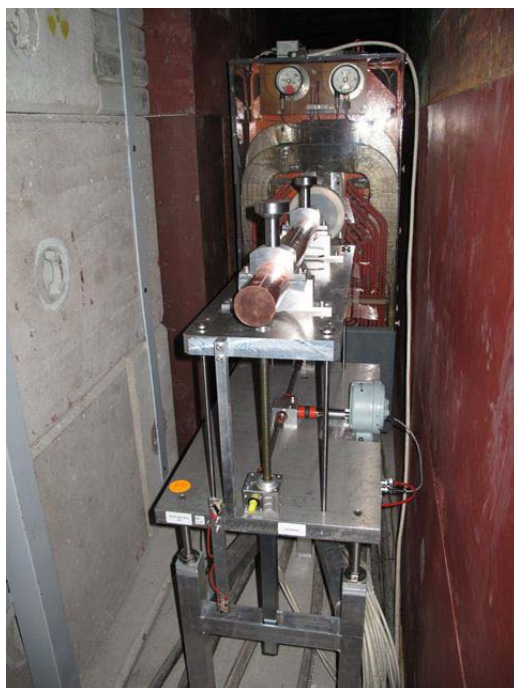
Figure 47: H4IRRAD copper target on a movable table [53].
