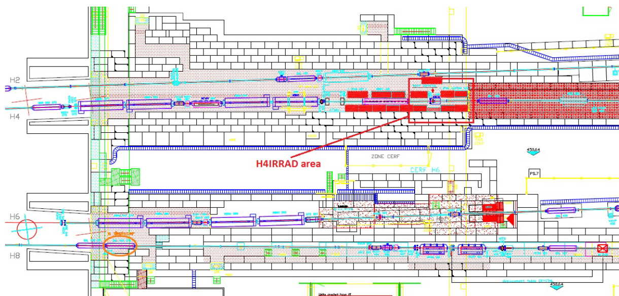
Figure 33: Layout technical drawing of a relevant part of the North Experimental Area with H4 beam line before H4IRRAD refurbishment [44].
