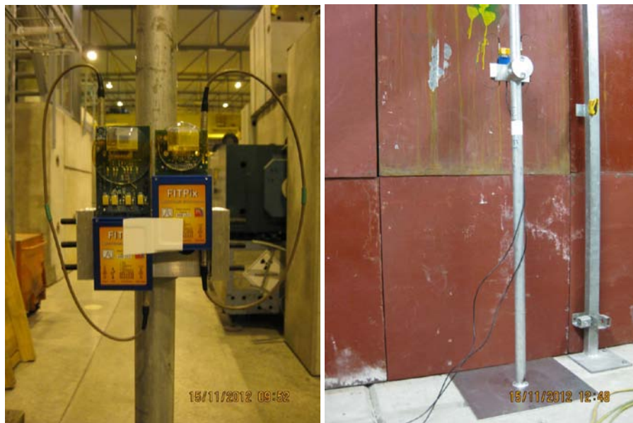
Figure 61: A detail of the aluminium support/holder with attached MPX and TPX detectors (left) and its position during measurements behind the beam dump (right).
