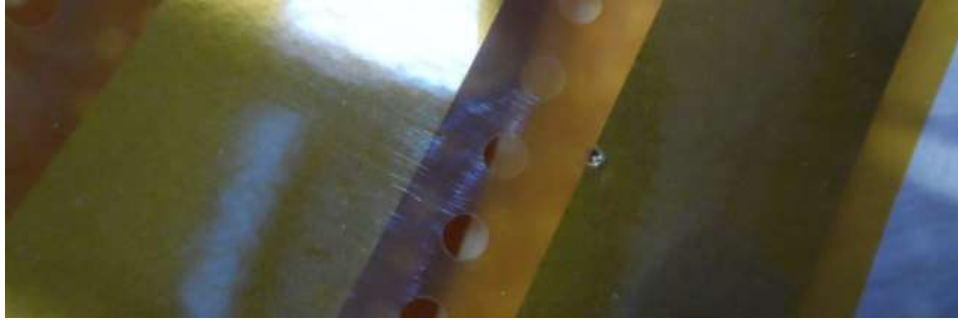
Figure 16: Perforated Polyimide film below the QH circuit that was detected during a HV test.
