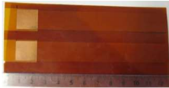
Figure 3: LHC quench heater terminal with cut-out of the Polyimide coverlay, so the quench heater power supply can be soldered to the heater trace.
