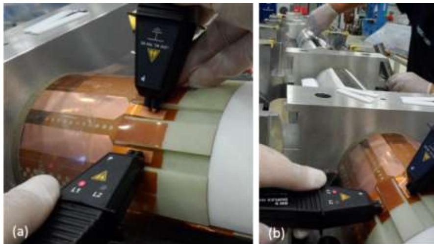
Figure 13: four-point resistance measurement of a quench heater circuit before impregnation with DLRO 10 handspikes.
