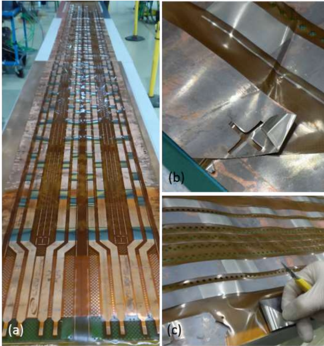
Figure 11: (a) Visual inspection of the QH T8000005/006 without large visible defects. (b,c) Delamination of the 304L foil from Polyimide film and thick oxide scale on the Cu coating of the heaters T8000003/004.
