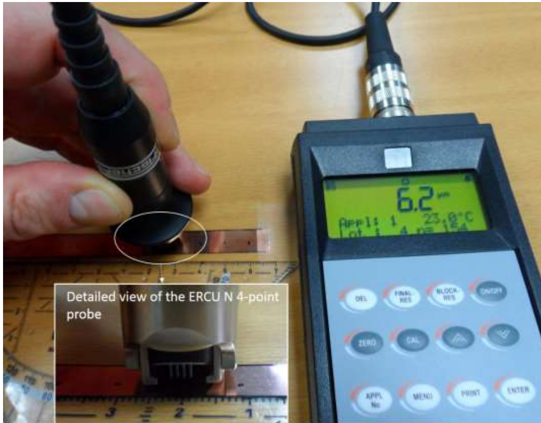
Figure 22: Cu coating thickness measurements with the Fischer SR-Scope RMP30-S tester in combination with the Fischer ERCU N four point probe.
