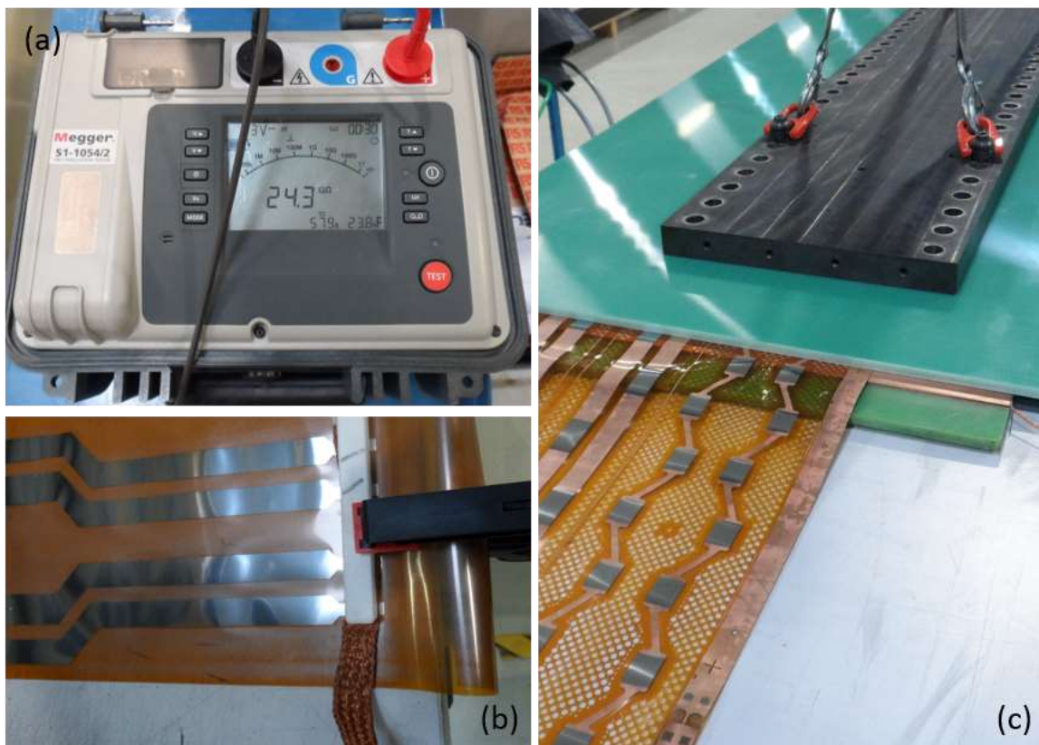
Figure 15: (a) The Megger S1-1054/2 insulation tester used for the dielectric measurements. (b) Connection of the tester to the QH terminals. (c) The test setup with additional weights.
