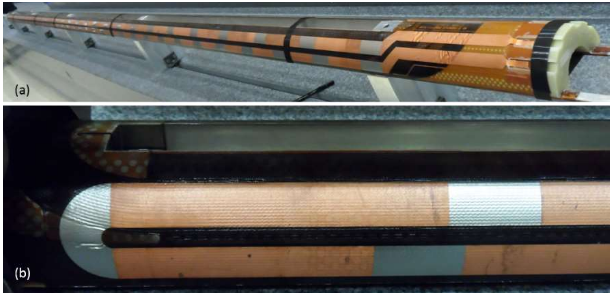
Figure 6: (a) Photograph of a quench heater installed on a 5.5 m long 11 T Nb 3 Sn coil. (b) Detailed view of the Cu plating pattern and circuit return end.
