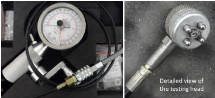
Figure 29: PAT handy adhesion tester in accordance with ASTM D4541 with the testing head for \varnothing 5.7 mm studs.
