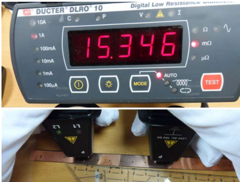
Figure 21: Four-point resistance measurement of a 10 mm wide, 160 mm long Cu coated sample, using a DLRO-10 with duplex handspikes.
