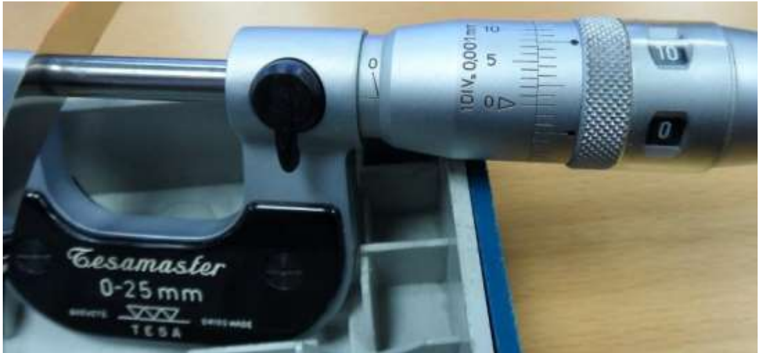
Figure 18: Measurement of the stainless steel foil thickness with a Tesamaster micrometre.
