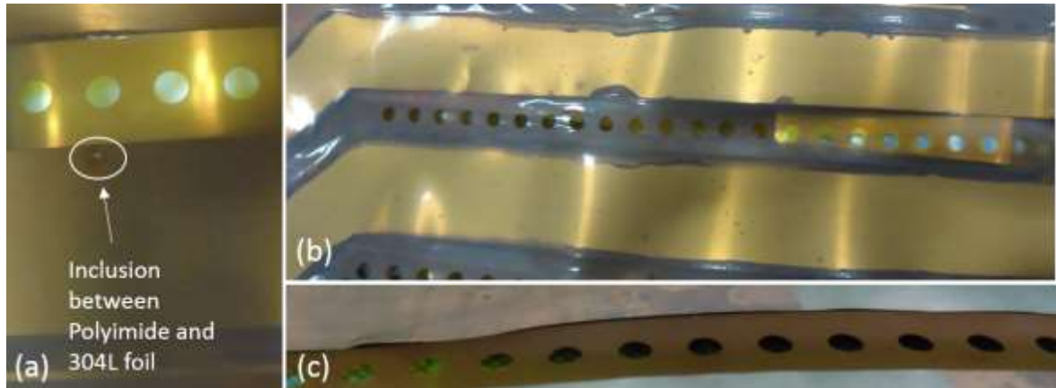
Figure 12: Heater circuit T8000003 and T8000004. (a) Inclusion between Polyimide film and 304L foil that may damage the Polyimide insulation. (b and c) Partially delaminated circuits.
