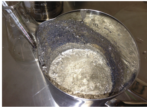
Figure 4.12: Crust of LBE oxide
