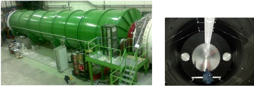
Figure 17: Left: the RICH vessel installed in the NA62 cavern. Right: the beam pipe seen from inside the RICH vessel; the entrance window and the location of the PMTs disks can clearly be seen.
