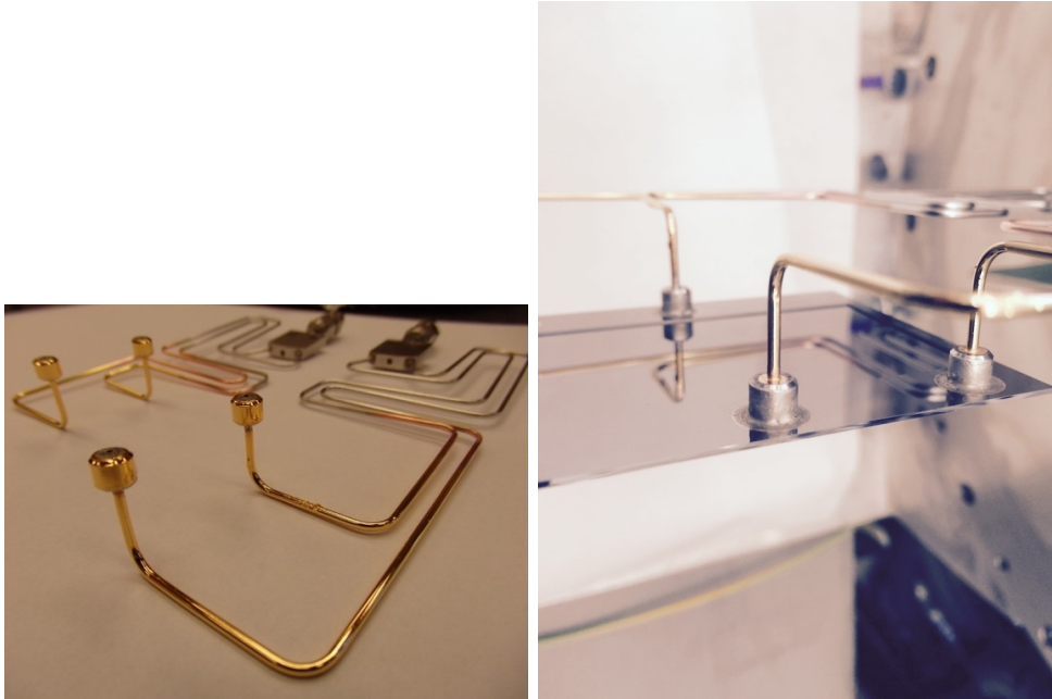
Figure 7: Left: Au-plated KOVAR connectors with an underlying layer of Cu. Right: Brazed connectors on the cooling plate of GTK_5.
