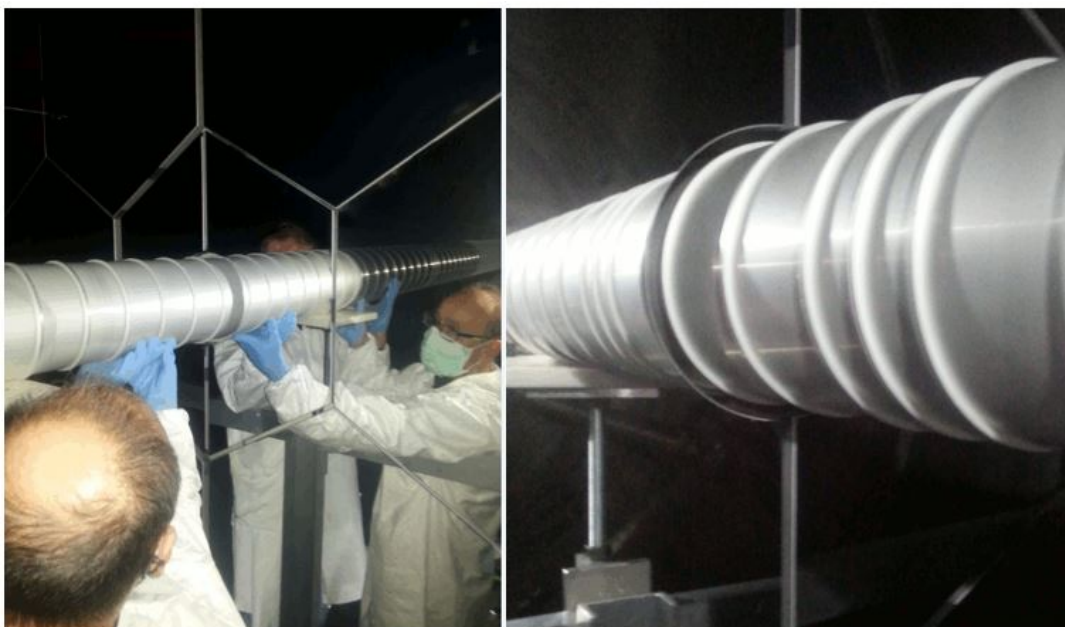
Figure 22: Left: Re-installation of the beam pipe through the mirror system. Right: Detail of the beam and the central mirrors.
