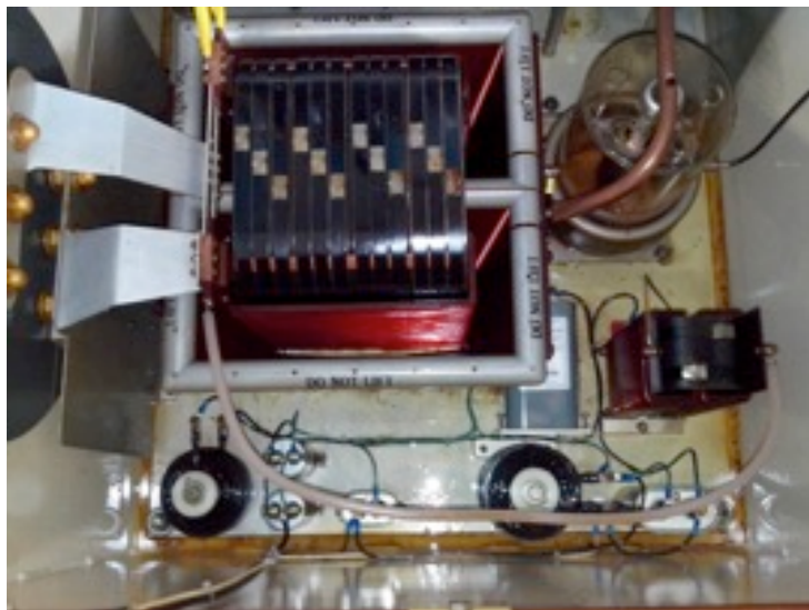
Figure 3.4: The klystron tank, hosting the pulse transformer and the capacitive divider 10,000:1 (for the measurement of the input klystron potential, V_k , on the top right of the picture).
