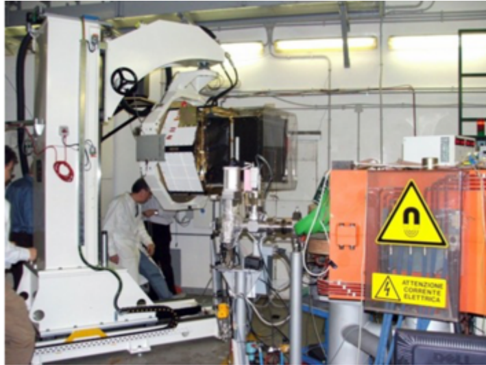
Figure 1.29: The AGILE gamma astronomy scientific payload installed on its dedicated movement system during the November 2005 dedicated calibration with the BTF tagged photon source.
