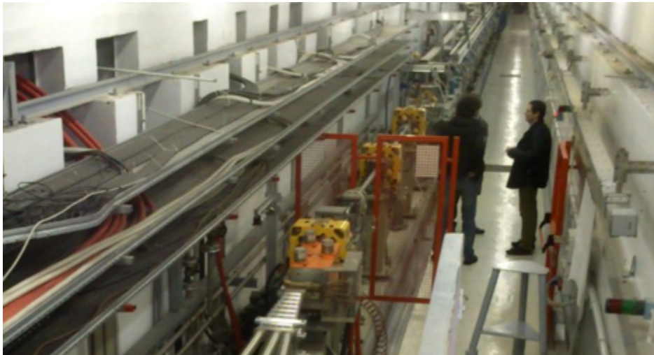
Figure 3.11: View of the LINAC tunnel from the three-way switch-yard, with the two pulsed magnets driving the beam towards the BTF line (3°, yellow dipole, more precisely a modified quadrupole) and the spectrometer line (6°, orange dipole), towards the LINAC (top of the picture). In between, a \approx 15 m drift, with four quadrupoles (yellow). In the upper part of the picture, the passageways towards the parallel modulator tunnel for cables, pipes and waveguides, is visible.
